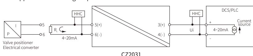
Note: HHC (HART Hand Held Communicator) cannot be used simultaneously on the input side and output side
