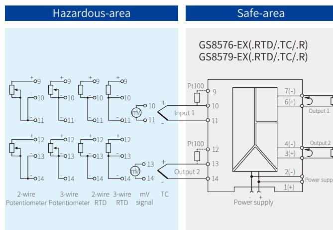
Note: a) GS8576-EX only contains input1, output1, output2;
