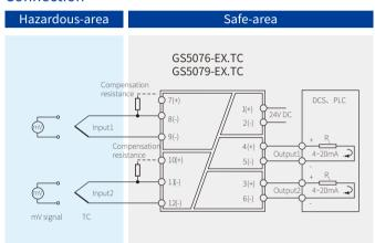
Note: a) GS5076-EX.TC only contains input1, output1, output2.
