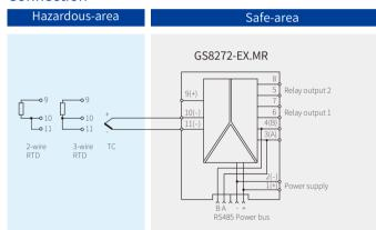
Note:a)Use normal terminals when RTD input; Use CJC terminals when TC input; b)Bus terminal is optional.
